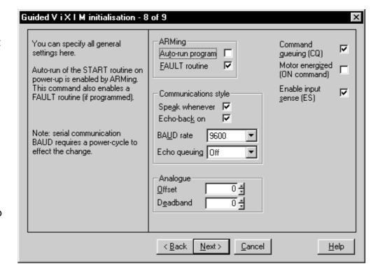
Press 'Next' to complete the setup process and to generate a setup program.
